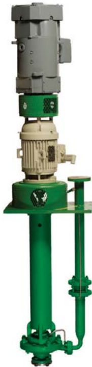
Piggy-back arrangement saves tank space by coupling DC motor with dual-shaft AC motor
